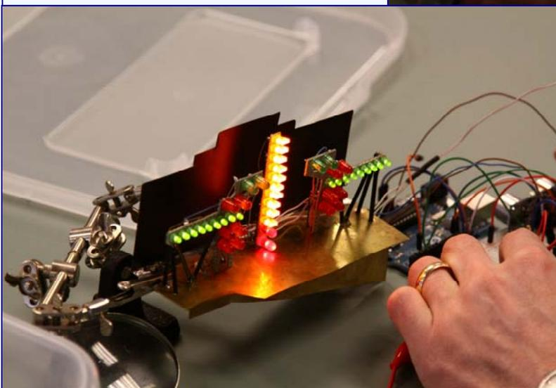
(Left) This is a breadboard LED miniature of the landing light system used on aircraft carriers which provides the pilot a stabilized visual glide slope position indicator. **Dan Klink** will place this on a 1:96 carrier!!!
