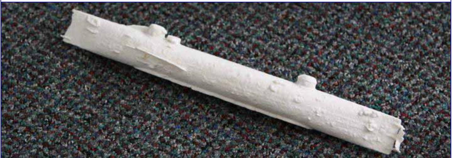
multi-billion point data cloud created with a precision laser scanning the real sub and then printing that data with a 3 dimensional printer. The model is about one foot long and shows to exact detail
