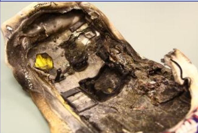
Twenty two attended the August meeting where LiPo battery safety was amply illustrated by the burned out hulk of a fast electric where the skipper had plugged a 2S and a 3S battery together in parallel, a huge no-no. Never parallel connect two dissimilar batteries!
