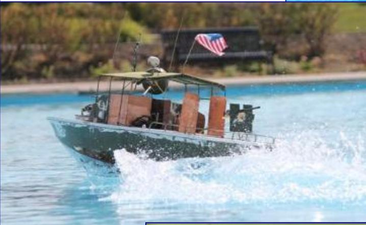
complete replacement of wiring, speed control, with battery conversion to LiPo and reballasting with \$2.60 worth of pennies. Displaying more than adequate power, only 385mah of the 4200mah capacity was used in 25 minutes of running!
